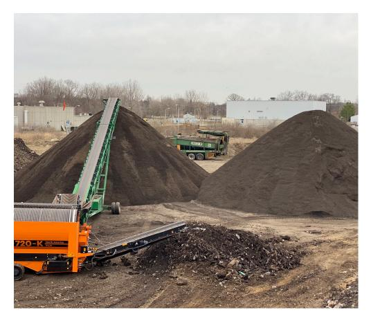
Spurt Industries' screening plant, where compost is screened, creating a better finished product and removing clumps in the soil. The equipment also separates and removes large pieces of wood that did not fully decompose and filters out contaminants like plastic and metal. Courtesy of My Green Michigan.
